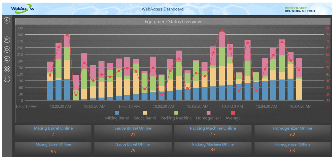
Figure 2 - The Dashboard Viewer shows designers how screens will look on remote viewing devices such as small-screen PCs and tablets.
