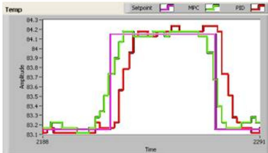
Figure 4. Comparison of an MPC Controller with a PID Controller Running on Two Temperature Chambers
